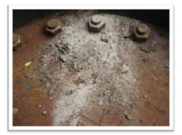
Cover plates over manholes should be removed and cleaned. All manholes covering ballast tanks must not have any evidence of water leaking through.
