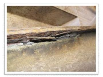
Sheet rust behind side frames may extend to upper reaches of frames. Check frames as high as possible particularly at the turn of the frames and in areas behind bent or damaged sections.
