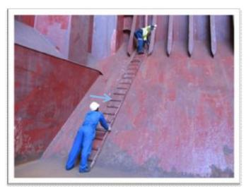
The ladder can be moved and braced at the bottom as the man on the hopper side cleans and checks behind frames
