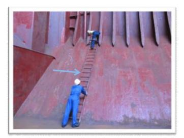
The man at the top should have a paint scraper to remove sheet rust from behind the frames
